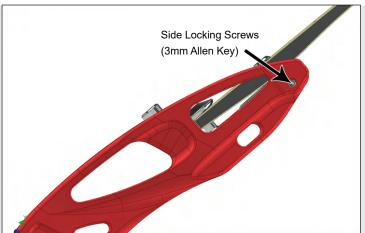
Alignment adjustments are best made while the bow is strung and after tiller and poundage has been set.
