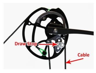
The purpose of a draw stop is to control the point at which the cam stops rotating. As you approach full draw, the cables come into contact with the stop. (See image). If the draw stop was moved slightly further back, the cam will rotate further, and 3 things happen.
